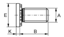
Head diameter E= 7.5Head height K +/-0.02 = 1.20Hole diameter +0.1= 4Length B +/-0.4= 30Male thread A= M4Min distance to edge= 9.5Tightening (N m)= 2.9
